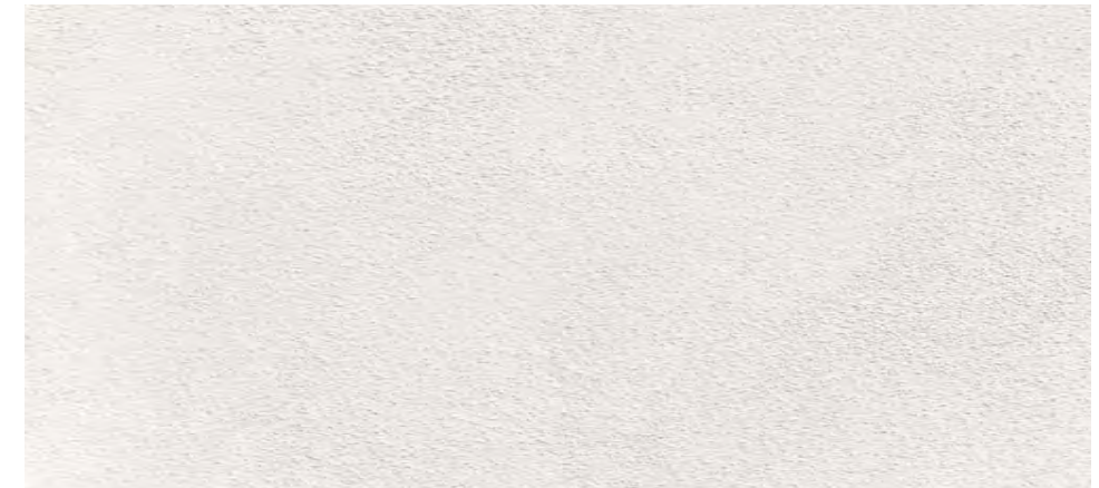
Painted Stucco (Exterior walls and soffits)
